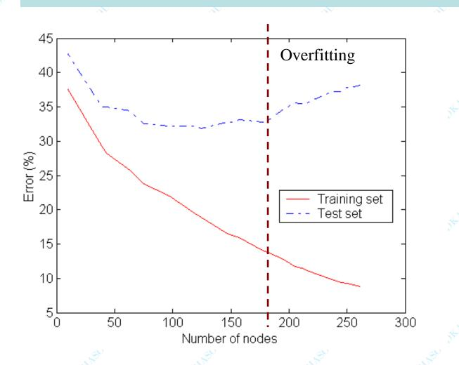
Underfitting: when model is too simple, both training and test errors are large
